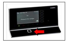
The KABA wall clock (TCD) has a built-in proximity ID reader which allows the employee to simply scan their all campus ID card in front of the reader to clock in/out. (Follow the onscreen instructions)
